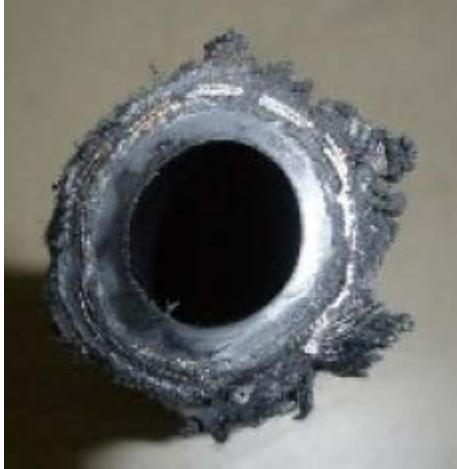
Figure 8. Cross-section of 12.7 mm ID fuel hose from a B20 unit.
