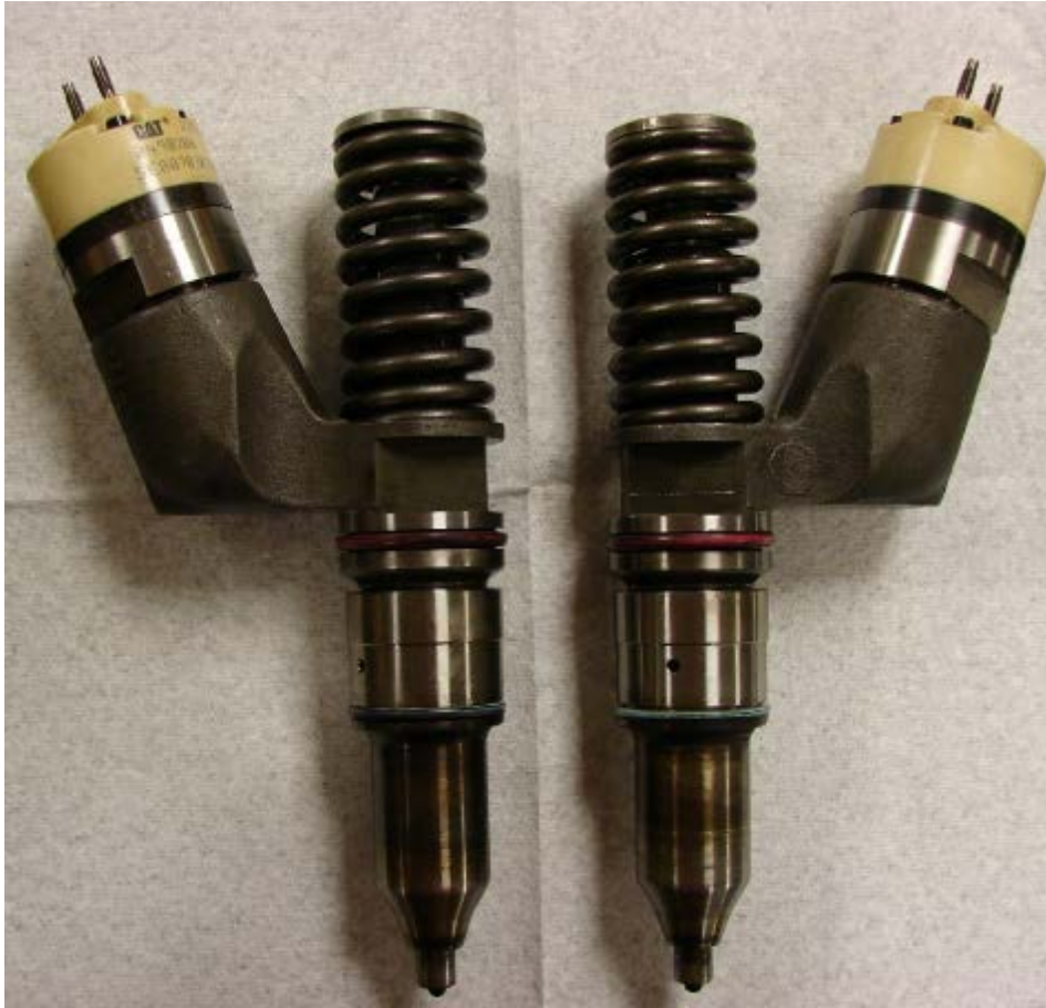
Figure 10. Biodiesel (left) and ULSD (right) injectors showing no discernable differences.
