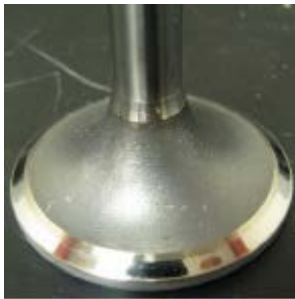
Figure 9. Cleaned intake valve from a B20 unit showing minimal wear.
